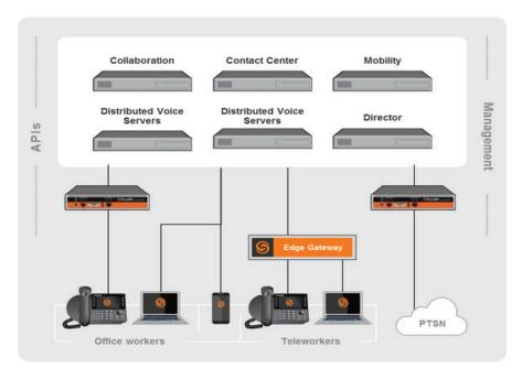
Companies can trust ShoreTel Connect ONSITE to provide secure connections to remote and teleworkers. The ShoreTel Edge Gateway provides VPN-free access via the WebRTC API and the Connect web collaboration app.
